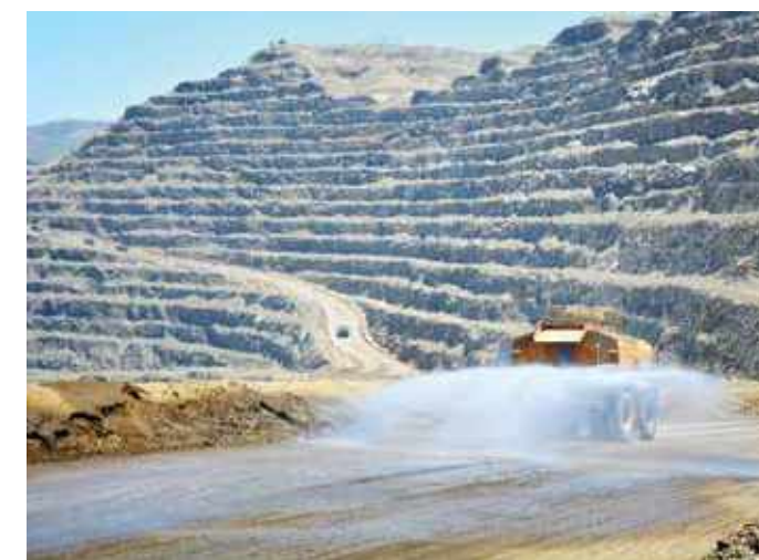
Dust Control Measures, Candelaria, Chile
